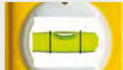
Vertical vial – for vertical measurements.
