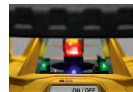
LED ASSIST system with indicators.
