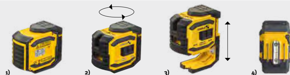
1) Park position. 2) Housing can pivot 360° inside the U-shaped housing. 3) The height of the laser can be adjusted thanks to the extendable foot. 4) Rear: rare-earth magnets with V-groove.
