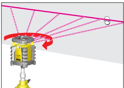
Laser planes can also be set up in advance by this method.
