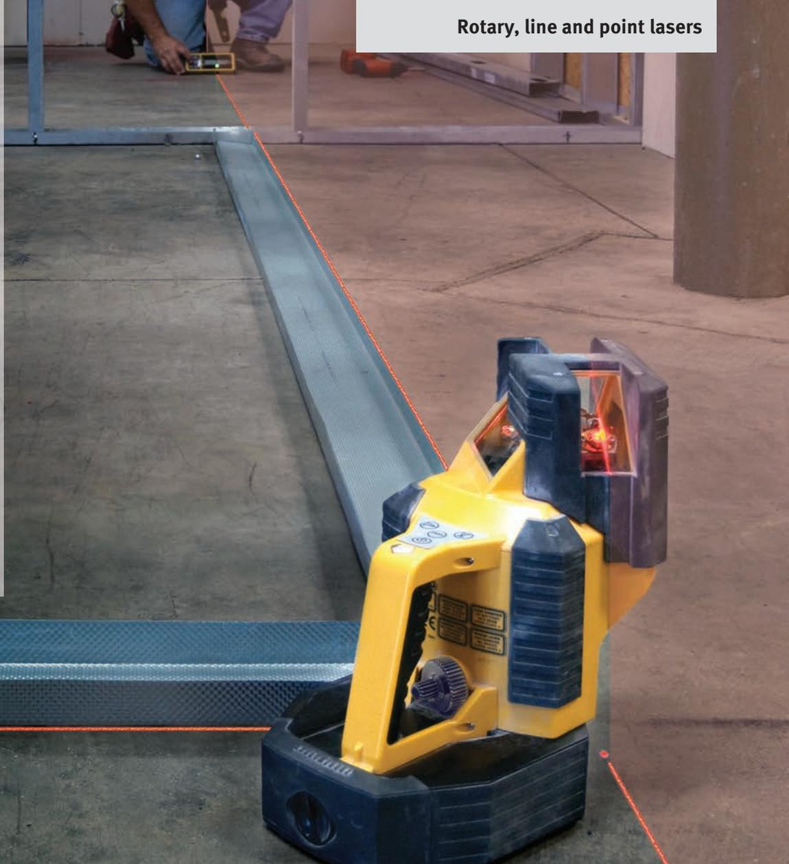
**AUTOALIGNMENT** for automatically transferring layout lines and creating right angles
